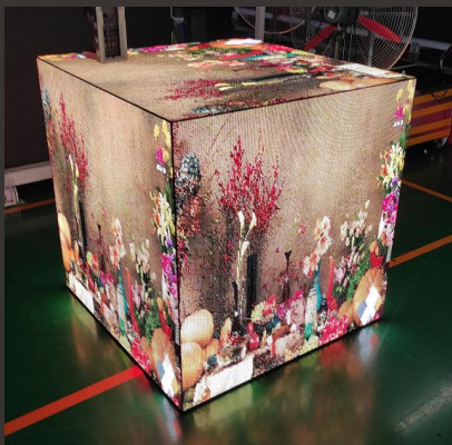
b. LED cube. One side cutting cabinet is only available to achieve the LED cube.
